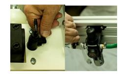
**Step 5**. Thread the sump back onto the filter housing by hand. Tighten with the SW4 filter wrench until it stops. Do not over tighten
