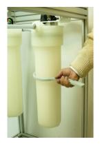
**Step 6**. Turn on the air valve. Vent air through the bleed valve as the filters fill. Close the bleed valve once all the air has been removed. The system is ready for normal operation
