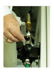
**Step 2**. Install Filter Klear hoses into sides of fountain solution tank, allowing space between hoses for circulation
