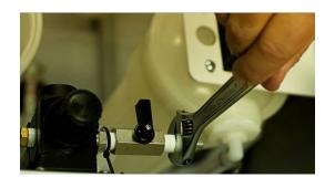
**Step 6**. Open the Air Bleed Valve and vent the air as the filters fill. Once all the air has been removed, close the vent. The system is now ready for normal operation
