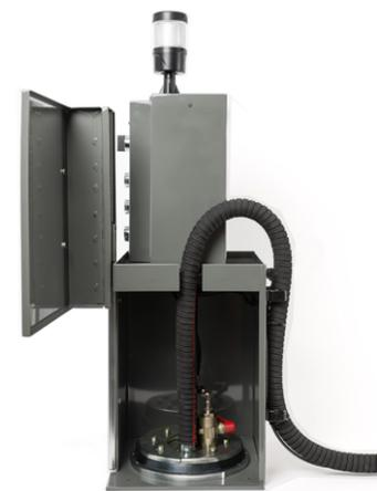
Ink can change outs can be completed in seconds and color sequence changes quick and simple with the use of a quick release pin allowing the wet end components (follower plate hose and manifold) to remain together easily moving them from unit to unit
